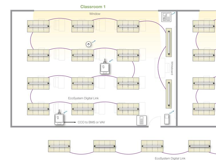
**Note:** The occupancy sensors in the classroom also communicate with the hallway PowPak, ensuring that the corridor lighting remains on when the classrooms are in use.
